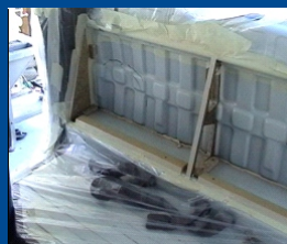
Preparation for application of Polyurethane lining in a Motor Vehicle Speaker enclosure.
