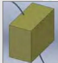
Electrical cable passing through thermal insulation
