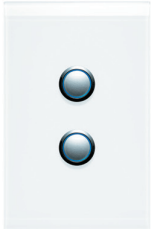
4062PBL, PW Push-button Switch, 2 Gang, Push-button, LED, Pure White, 20A/16AX, 250V a.c.
