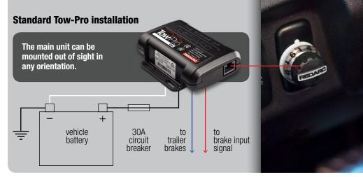
The remote head control is mounted in the dash of your vehicle and the electronic module is mounted out of sight, making the Tow-Pro ideal for vehicles fitted with knee or lower leg airbags.
