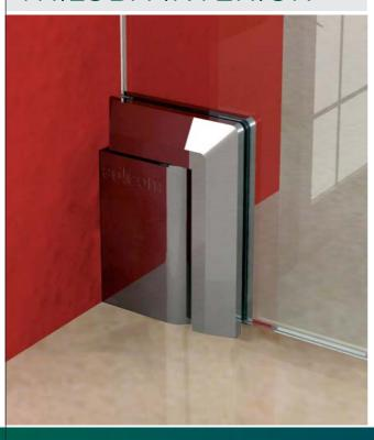
A unique alternative to the conventional in-ground Hydraulic Door Closer, **Triloba** is surface mounted and incorporates the hydraulic closer within the patch fitting. A range of additional components make fully frameless glass entrances possible with glass up to 120kg and 1200mm wide.
