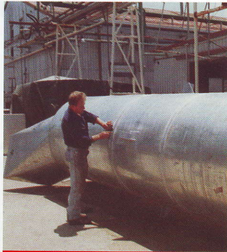
CIRCULAR SILENCER FOR DUST COLLECTION FAN DISCHARGE
