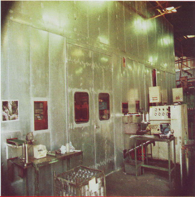
PUNCH PRESS ACOUSTIC ENCLOSURE FOR FASCO AUSTRALIA 13 M x 4.5 M x 5.5 M H
