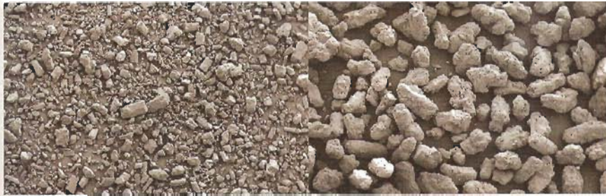
ABOVE ▲ Left side of photo shows store-bought (in the box) baking soda powder. Right side shows blasting soda, which is coarse in size with minimal fines. Original magnification 30X.
