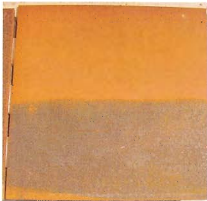
ABOVE ▲ Figure D. Plate was sandblasted on the top half and sodablasted on the bottom half. After two months the upper sandblasted area has considerable rusting while the lower sodablasted surface shows little rusting.
