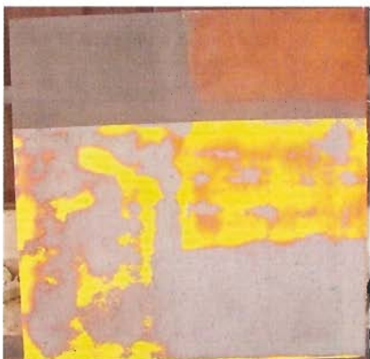
ABOVE ▲ Figure F. Left top of plate was sodablasted and left untouched. Upper right was originally sandblasted. Bottom was sandblasted then painted with a primer, intermediate layer and topcoat. It was later spot sodablasted down to previously sandblasted metal exposing original anchor profile.
