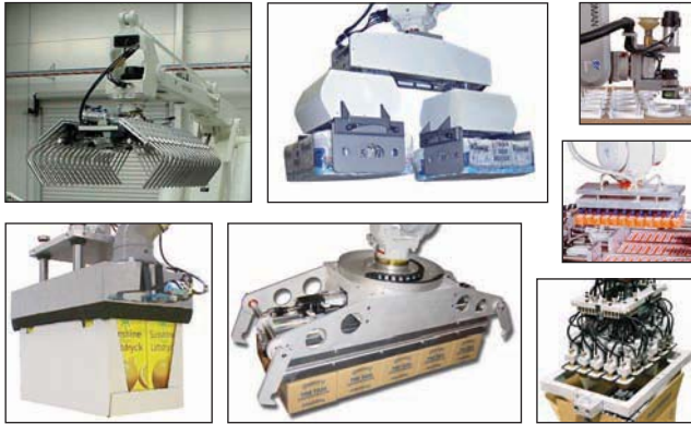
Some of the end-of-arm grippers designed/integrated by RA
