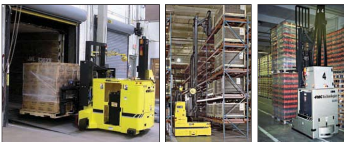
Trailer Loading via end or side access
