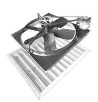
The heart of the Breeze Power System is the large, quiet-in-roof fan. The fan creates a powerful updraught that instantly sets the air inside your home in motion, causing it to flow towards the fan, through the ceiling shutter and into the roof space.
