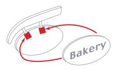
Aluminium arm to suspend the sign is bonded between the two sign faces with 3M Scotch-Weld EPX Adhesive.
