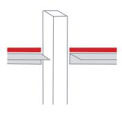
Sign face is bonded to metal stiffeners using 3M VHB Tape.
