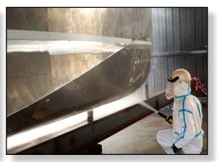
Wet abrasive blasting is ideal for preparing any type of surface prior to repainting or re-coating, and it effectively removes old layers of paint and industrial coatings, and can also be used to remove corrosion, rust and other contaminants from many different types of materials and surfaces.
