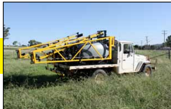
18.5m Manual Fold Truck Mounted SmartBoom. Custom built to suit Isuzu 300 Truck.
