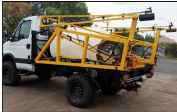
14m Ute Mounted SmartBoom. Custom built to suit short tray length.
