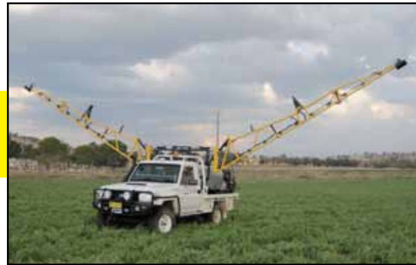
21.5m Manual Fold, Hydraulic Wing Tilt Truck Mounted SmartBoom. Custom built to suit Iveco Daily Truck.
