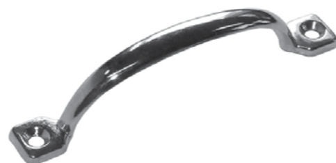
Grab Handle CLLH-1048 Aluminium diecast handle; hole centres 100mm or 135mm;
