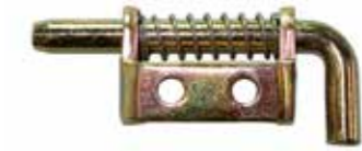
H00117-2 Zinc plated steel; 6mm dia. Pin; Dimensions: 30mm x 10mm; Left & Right Hand available (LH shown)
