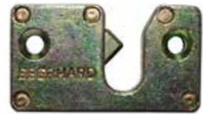
561 Die cast slam latch; uses 0.31 inch dia rod; load rating 100lbs
