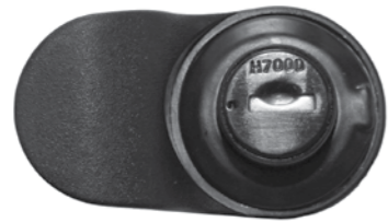
626 1/4 TURN SLAM LATCH; key locking; water resistant; black plastic with stainless steel dust shutter; 90 degree rotation
