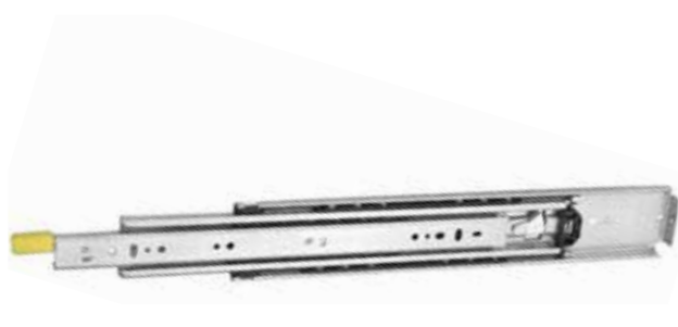
9308 Drawer Slide; 226kg load rating. Lock-in/ Lock-out. Non-disconnect; AVAILABLE LENGTHS: 10" - 60" (254-1524mm)
