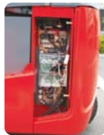
The controller is securely housed in the left side of the frame.
