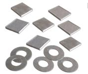
Silicone Bonded Mica is a high temperature insulation board which exhibits very good mechanical strength and excellent electrical insulation properties. This board is utilised in applications with temperatures up to 500°C and is often employed for the manufacture of heat or arc shields, as well as high temperature stand-off or brake grid insulators. Silicone Bonded Mica is silver/grey in colour and available in a wide variety of thicknesses as well as custom machined or cut components.
