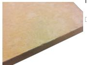
Millboard in a large range of thicknesses. This excellent thermal insulation material exhibits very low thermal conductivity and resistance to temperatures up to 1000°C. Manufactured from a precise blend of mineral fibres with inorganic binders, Millboard is free of ceramic fibres and is often used for high temperature gaskets, furnace linings, boiler insulation, oven linings, thermal shields and behind splashbacks.
