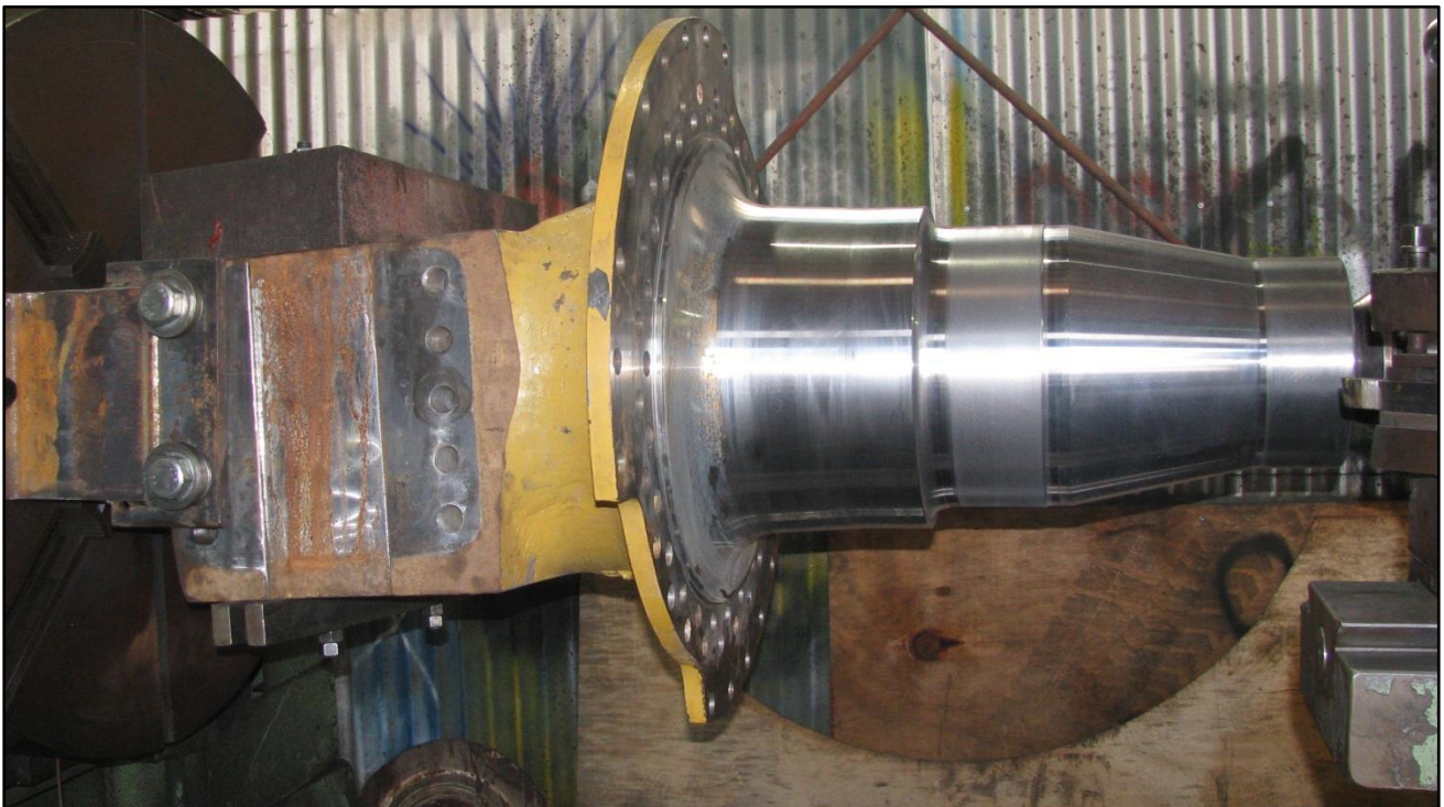
789 Front Wheel spindle – bearing reclamation
