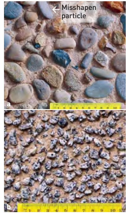
Figure 9 [a] Large river gravel (nominal 50-mm) containing misshapen particles seeded onto surface [b] 10-mm crushed aggregate mix
