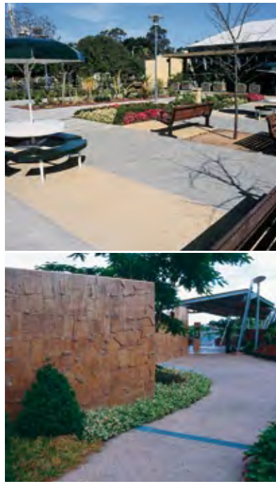
Figure 2 Matrix may be coloured to match the aggregate colour
