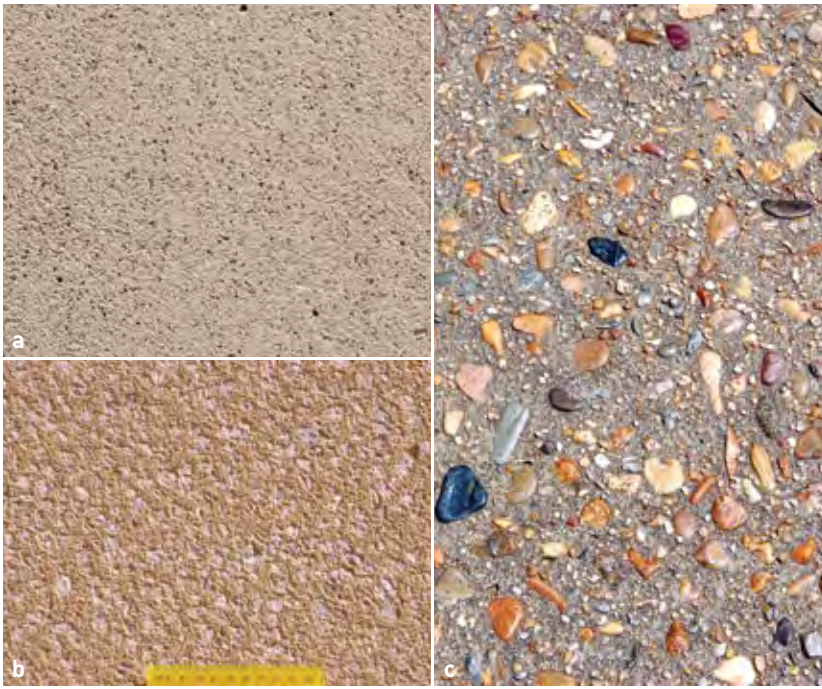
Figure 32 Grades of abrasive blasting
