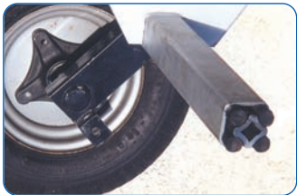
Axle with integrated rubber suspension
