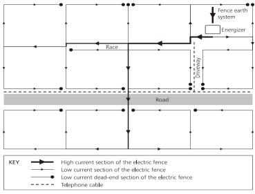
The ideal way to set up your electric fence is to feed the power out from the energizer in a 'star' fashion, with no closed loops and low currents in parts of the fence that closely parallel phone lines.
