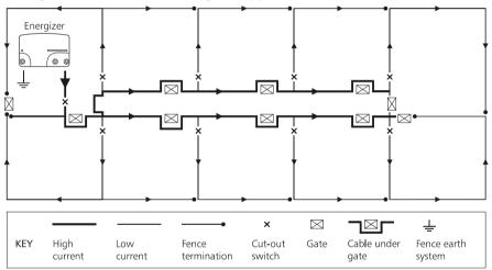
It is important to consider how the fencing plan will affect telecommunications. Avoid a long leadout running adjacent to telephone lines. If this is unavoidable, feed the power to the fence in a 'star' fashion with no closed loops. This will ensure low currents in the sections of fence that are in close proximity to telephone lines. See *Telecommunications interference* on page 27.
