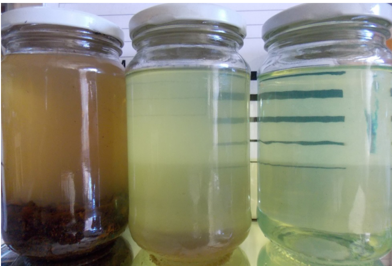
Samples showing fuel quality improvement during the cleaning process.
