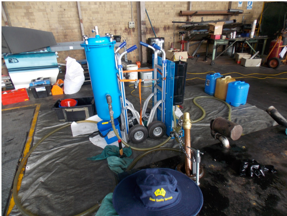
DQS-90-TCM (right) and DQS-120-TSF (left) as set up for operation. The rigid suction lance can be seen inserted into the tank port in the fore-ground.
