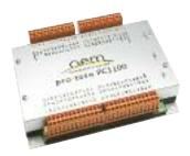
The provides PCII00 Programmable Controller provides flexibility by incorporating universal inputs that can be analogue or digital. Added to the existing I/O configuration this added flexibility ensures that the PCI 100 fits the application exactly.
