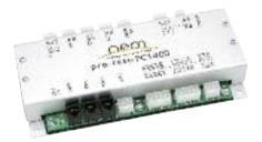
The **Droless** PCI400 Programmable Controller provides an assortment of I/O interfaces for those difficult applications where equipment interfaces are not always straight forward. High and low side digital inputs, relay and transitor driver outputs, differential and single ended analogue inputs. The PC1400
