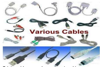
Printer, video, sound, power, networking, camera and monitor cables. USB. parallel. VGA. DVI. HDMI. Ethernet, PSU splitters, 3.5 stereo & PS2 adaptors.
