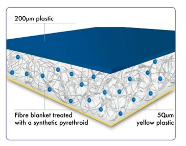
Trithor is impregnated with deltamethrin and laminated top and bottom with a rugged plastic membrane. The unique fibre blanket within Trithor adds to its durability and effectiveness. The non-woven blend of fibres within Trithor, in addition to holding the deltamethrin crystals so they remain ever ready to kill and repel termites, is also structured to prevent termites penetrating.
